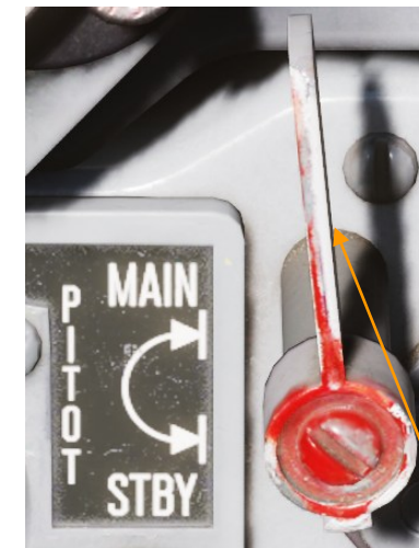
Figure 34: Pitot selection lever
