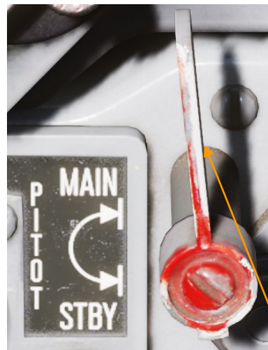
Figure 34: Pitot selection lever
